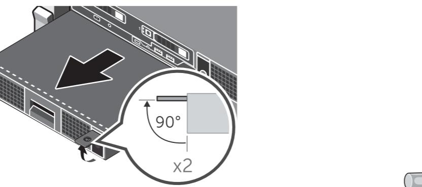
1. Use a Phillips #2 screwdriver to unlock the **Sled Release** lock.
