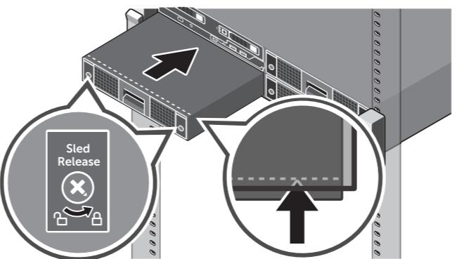
1. Slide the storage sled into the enclosure until the dotted line on top of the sled is not visible from the top edge of the bay and the sled clicks into place.
